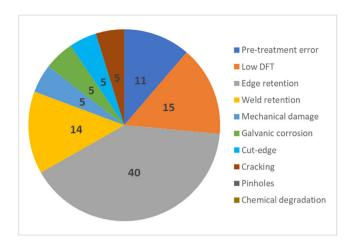
**FIGURE 4** Percentage distribution of root cause for corrosion on painted steel on topside oil and gas offshore installation. [Color figure can be viewed at wileyonlinelibrary.com]
