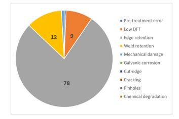
**FIGURE 6** Percentage distribution of root cause for corrosion on painted steel in ballast water tanks. [Color figure can be viewed at wileyonlinelibrary.com]
