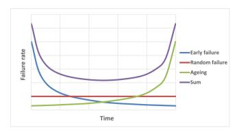
**FIGURE 1** The bathtub curve of failure rate as a function of time, applied to failure of a protective coating on a steel structure. [Color figure can be viewed at wileyonlinelibrary.com]
