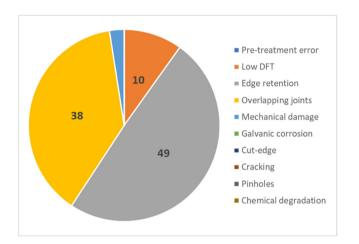
**FIGURE 8** Percentage distribution of root cause for corrosion on painted steel on bolted thruss work on a coastal steel bridge protected with a three-coat paint system. [Color figure can be viewed at wileyonlinelibrary.com]
