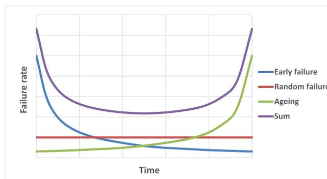
**FIGURE 1** The bathtub curve of failure rate as a function of time, applied to failure of a protective coating on a steel structure. [Color figure can be viewed at [wileyonlinelibrary.com](http://wileyonlinelibrary.com)]
