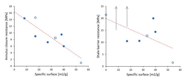
Fig. 10. Correlation plots between specific surface and annulus closure resistance (left) and shale barrier resistance (right). Open circular symbols (o) represent results from underbalanced tests. The open square symbol () represents sample F5 (c.f. footnote c of Table 2). The red dashed lines are linear trend lines.
