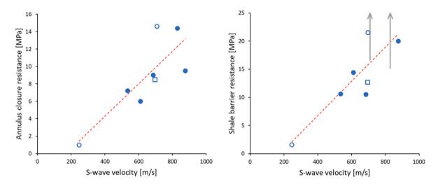
**Fig. 7.** Correlation plots between S-wave velocity and annulus closure resistance (left) and shale barrier resistance (right). Open circular symbols (o) represent results from underbalanced tests. The open square symbol ( $\Box$ ) represents sample F5 (c.f. footnote b of Table 1 and footnote c of Table 2). The red dashed lines are linear trend lines (not including sample F5).
