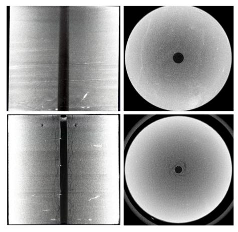
Fig. 3. CT scans of the O1 sample, before the test (upper row; without casing) and after the test (lower row; with casing in place).
