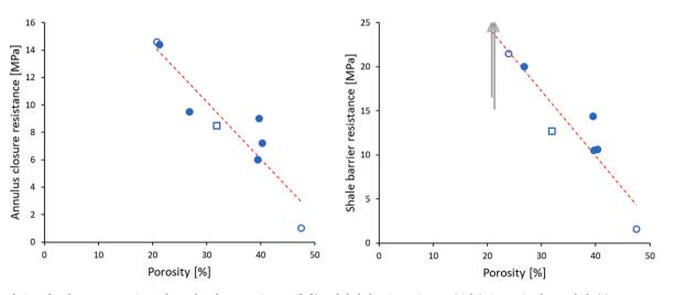
Fig. 5. Correlation plots between porosity and annulus closure resistance (left) and shale barrier resistance (right). Open circular symbols (o) represent results from underbalanced tests. The open square symbol (
