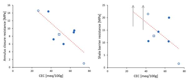
Fig. 9. Correlation plots between CEC and annulus closure resistance (left) and shale barrier resistance (right). Open circular symbols (o) represent results from underbalanced tests. The open square symbol ( $\Box$ ) represents sample F5 (c.f. footnote c of Table 2). The red dashed lines are linear trend lines.
