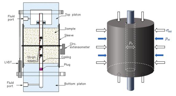
Fig. 1. Test cell configuration, sample, and pressures.
