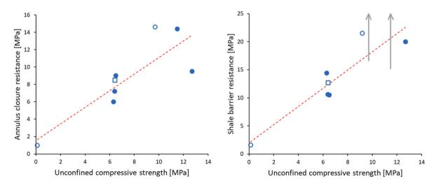
**Fig. 8.** Correlation plots between unconfined compressive strength (UCS) and annulus closure resistance (left) and shale barrier resistance (right). Open circular symbols (o) represent results from underbalanced tests. The open square symbol ( $\Box$ ) represents sample F5 (c.f. footnote e of Table 1 and footnote c of Table 2). The red dashed lines are linear trend lines (not including sample F5).
