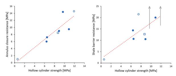
Fig. 4. Correlation plots between hollow cylinder strength (HCS) and annulus closure resistance (left) and shale barrier resistance (right). Open circular symbols (o) represent results from underbalanced tests. The open square symbol ( $\Box$ ) represents sample F5 (c.f. footnote c of Table 2). The red dashed lines are linear trend lines.
