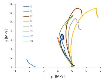
**Fig. 11.** p'-q plots from a CIU test for all materials, except F5. The O2 sample could not be stabilized at p' = 5 MPa, hence this test was run at a lower level. This has no consequence for the conclusion drawn from this plot.
