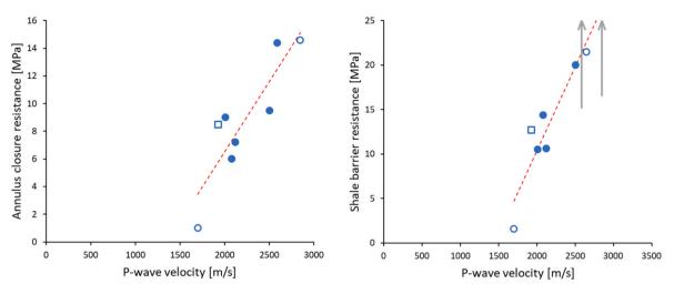
Fig. 6. Correlation plots between P-wave velocity and annulus closure resistance (left) and shale barrier resistance (right). Open circular symbols (o) represent results from underbalanced tests. The open square symbol ( $\Box$ ) represents sample F5 (c.f. footnote c of Table 2). The red dashed lines are linear trend lines.
