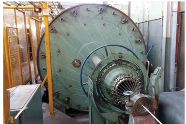
Fig 6: Planetary cabling machine for the cable conductor
