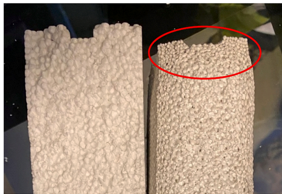
Fig. 3. Visual comparison of shrunken EPS material (top view). The heat affected test sample on the right is clearly smaller in size compared to the reference sample on the left. The red circle on the right highlights the area where shrinking is most distinct.
