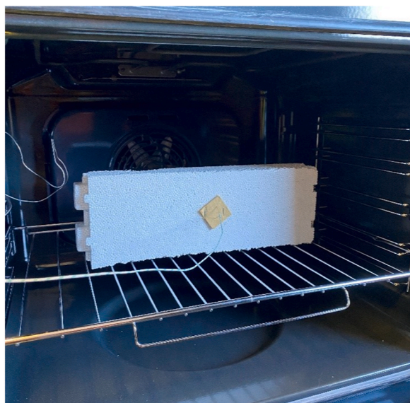
Fig. 1. Test setup used to determine the temperature range for structural change in the specific EPS material used in the main tests. The picture shows a sample of EPS material with a disc thermocouple attached to the side.
