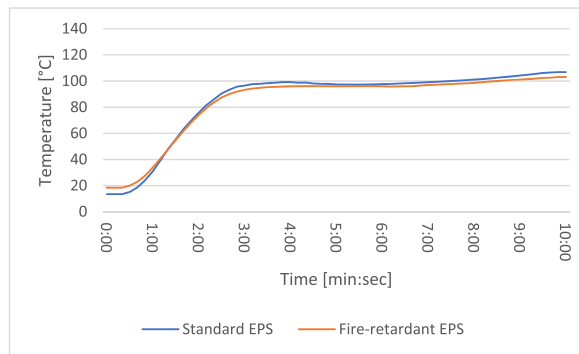
Fig. 20. Comparison of recorded temperatures for Tests 7 (single layer of gypsum covering standard EPS) and 8 (single layer of gypsum covering fire-retardant EPS).
