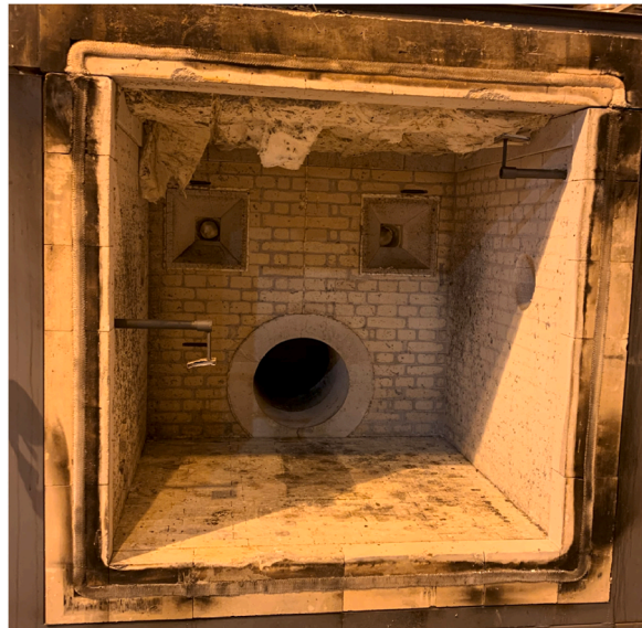
Fig. 7. Indicative fire resistance test furnace.
