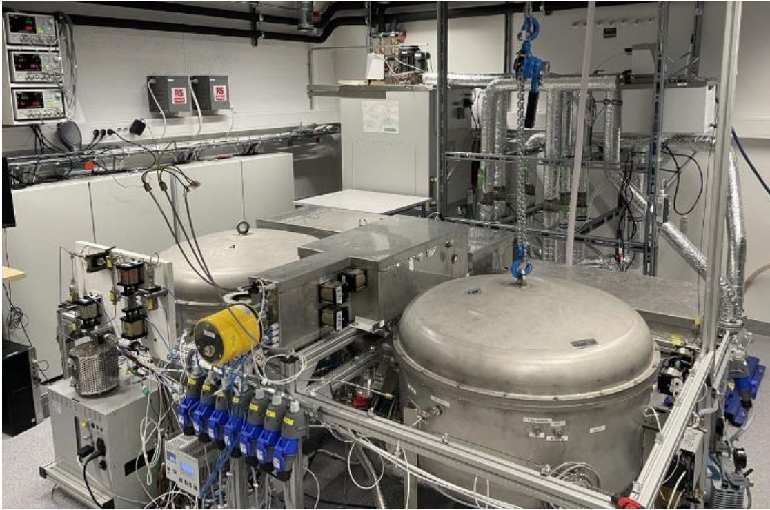
Fig. 2: A picture of two- capillary viscometer facility.
