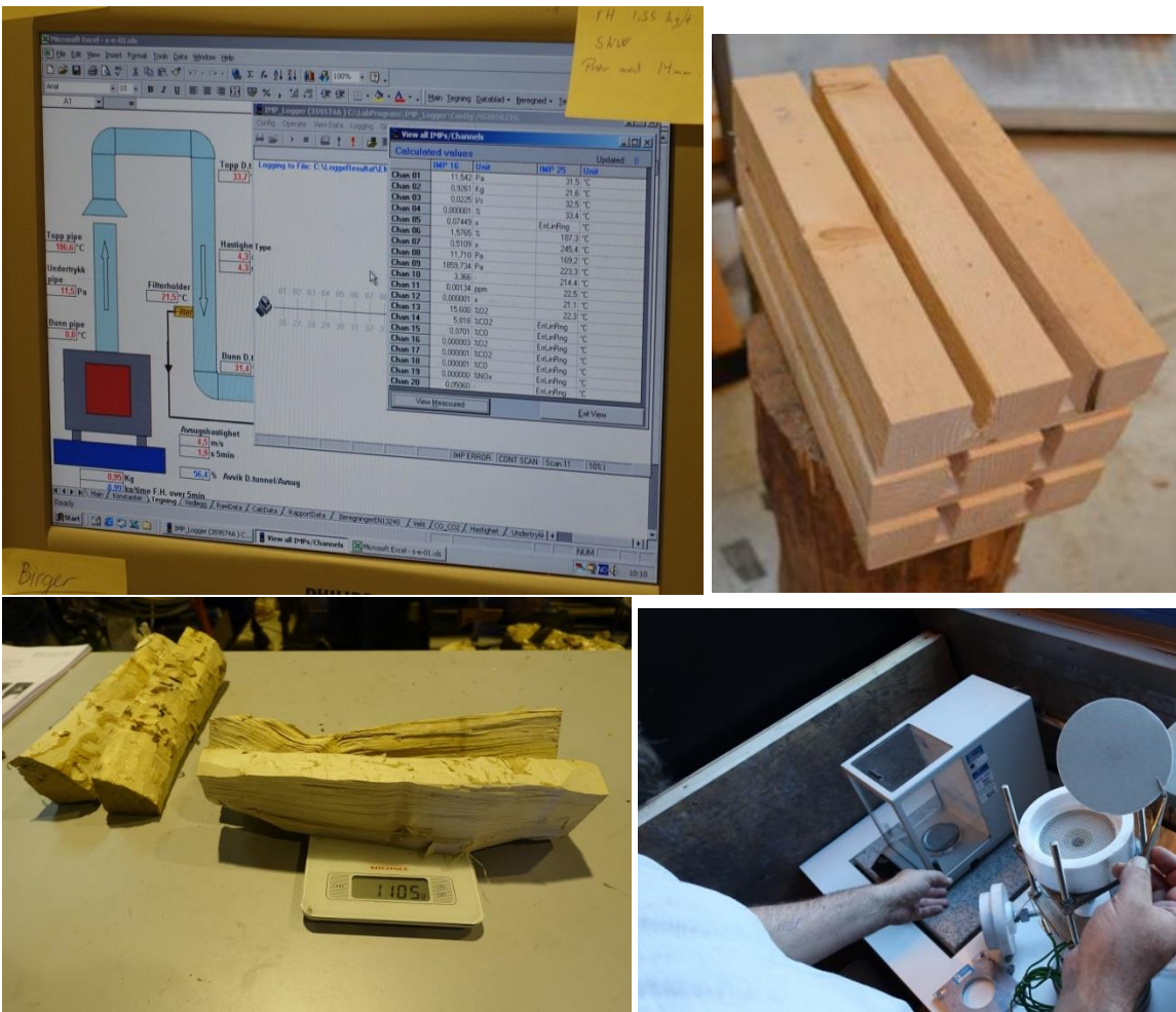
Figure 6: Experimental setup - software for data logging; spruce according to NS3058-59; birch without bark is used when performing tests according to DIN+; manual handling of filters for gravimetric analyses.
