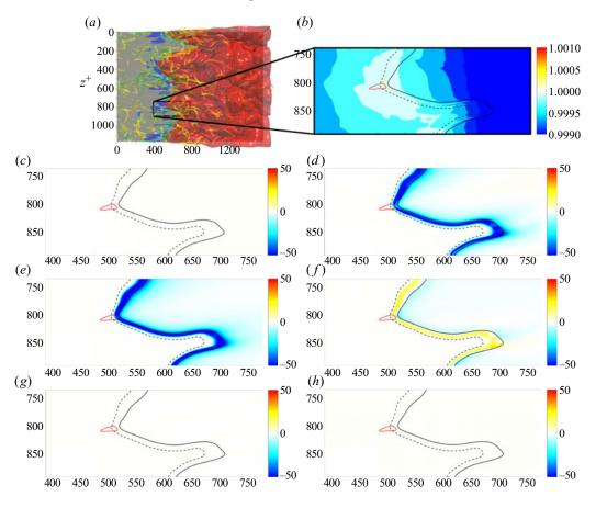
Figure 12. Instantaneous contours of (a) flame front and  $\lambda_2$  vortex, (b) normalized pressure and (c-h) budget terms of the pressure transport equation in an x-z plane. The dashed and solid black lines in (b-h) denote the isosurfaces of c = 0.01 and c = 0.7, respectively. The red solid line indicates the isoline of  $u = 0 \text{ m s}^{-1}$  (backflow region); (b)  $p/p_0$ , (c)  $T_0$ , (d)  $T_1$ , (e)  $T_2$ , (f)  $T_3$ , (g)  $T_4$ , (h)  $T_5$ .
