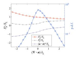
Figure 9. Normalized density-weighted  $S_d$ ,  $S_f$  and  $u \cdot n$  conditionally averaged on the flame curvature in the buffer layer. The blue line denotes the p.d.f. of the normalized curvature.
