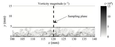
Figure 3. Instantaneous distribution of vorticity magnitude (s<sup>-1</sup>) of the turbulent flow at an *x*-*y* plane for the auxiliary DNS. The dashed line indicates the location of the sampling plane with  $Re_{\tau} = 360$ . The dotted line denotes the boundary layer thickness at x = 120 mm.
