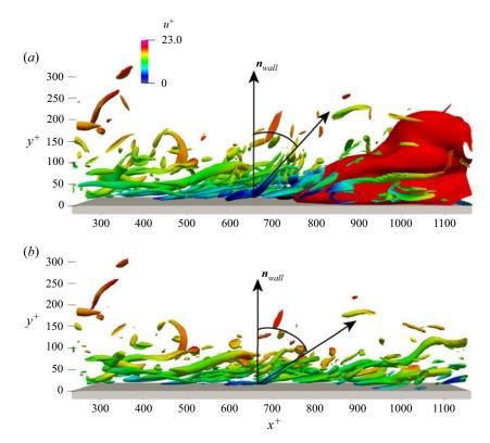
Figure 17. Instantaneous contours of turbulent boundary layer coherent vortical structures (represented by  $\lambda_2 = -6 \text{ s}^{-1}$  isosurface and coloured by streamwise velocity) for the (*a*) reacting and (*b*) non-reacting cases. The red isosurface denotes the flame front (represented by c = 0.7).
