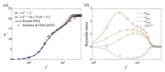
Figure 2. (a) Profile of mean streamwise velocity along with the wall-normal direction. (b) Profiles of Reynolds stress components along the wall-normal direction. Symbols denote the DNS data in Schlatter & Örlü (2010).
