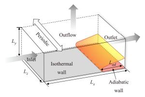
Figure 1. Schematic of the configuration.
