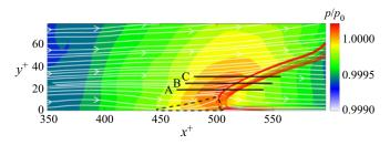
Figure 13. Instantaneous distribution of normalized pressure in a typical x-y plane with a flame bulge for the 3-D case. The white lines indicate the streamlines. The black dashed line and red isolines denote the backflow region and the heat release rate, respectively. Three lines are used to extract the budget terms of the pressure transport equation. The value of wall-normal distance is  $y^+ = 18$ , 24 and 30 mm for lines A, B and C, respectively.
