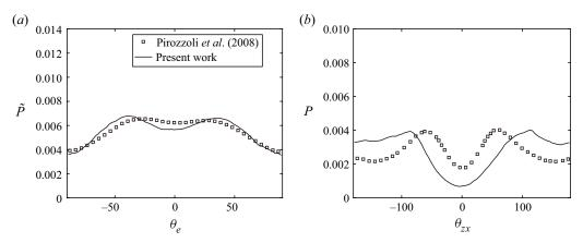
Figure 19. The p.d.f.s of the characteristic angles for the non-reacting case: (a)  $\theta_e$  and (b)  $\theta_{zx}$  in the logarithmic region. The DNS results of Pirozzoli *et al.* (2008) are also included.
