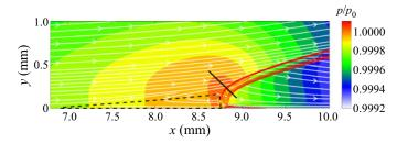
Figure 10. Instantaneous distribution of normalized pressure in an x-y plane with a flame bulge for the 2-D case with flashback. The white lines indicate the streamlines. The black dashed line and red isolines denote the backflow region and the heat release rate, respectively. The black solid line is used to extract the budget terms of the pressure transport equation. The length of the black line is 0.4 mm.
