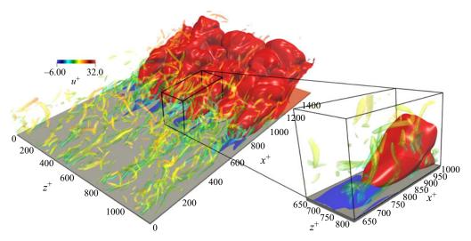
Figure 7. The instantaneous distribution of the flame front (represented by red isosurface) and the backflow region (represented by blue isosurface). The boundary layer turbulence (characterized by  $\lambda_2 = -6 \text{ s}^{-1}$ ) are shown and coloured by streamwise velocity.
