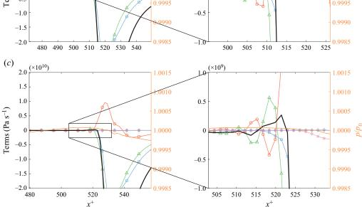
Figure 14. Budget terms of the pressure transport equation extracted from the black lines in figure 13: (a) line A, (b) line B and (c) line C.
