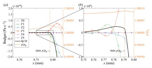
Figure 11. Budget terms of the pressure transport equation extracted from the black line in figure 10.
