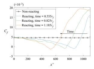
Figure 16. The profiles of mean skin-friction coefficient  $C_f$  along the streamwise direction for the reacting and non-reacting cases. The average is conditioned on the spanwise direction for the reacting case, and on time and the spanwise direction for the non-reacting case.
