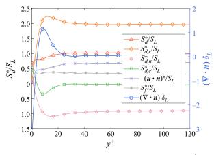
Figure 8. Conditional means as a function of normalized wall-normal distance  $y^+$  of the following quantities:  $S_d^*/S_L, S_{d,r}^*/S_L, S_{d,n}^*/S_L, S_{d,c}^*/S_L, -(\boldsymbol{u} \cdot \boldsymbol{n})^*/S_L, S_f^*/S_L \text{ and } (\nabla \cdot \boldsymbol{n})\delta_L.$
