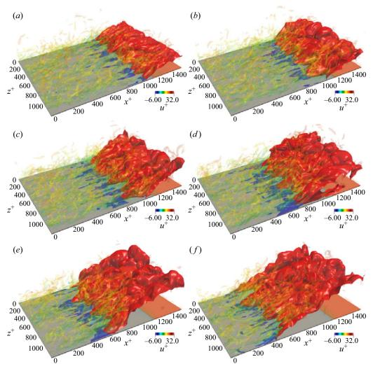
Figure 6. Temporal evolution of the premixed flame with the instantaneous distribution of the flame front (represented by red isosurface) and the backflow region (represented by blue isosurface). The boundary layer turbulence (characterized by  $\lambda_2 = -6 \text{ s}^{-1}$ ) is shown and coloured by streamwise velocity; (a) Time =  $0.21 \tau_f$ , (b) Time =  $0.435 \tau_f$ , (c) Time =  $0.66 \tau_f$ , (d) Time =  $0.90 \tau_f$ , (e) Time =  $1.14 \tau_f$ , (f) Time =  $1.38 \tau_f$ .
