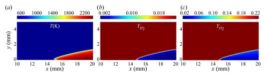
Figure 4. Distributions of (*a*) temperature, mass fraction of (*b*) hydrogen and (*c*) oxygen for the stabilized 2-D boundary layer flame.
