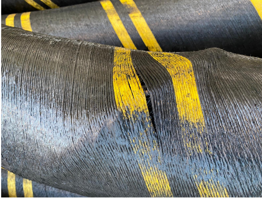
Figure 81: Probable birdcaging (Courtesy of TenneT)
