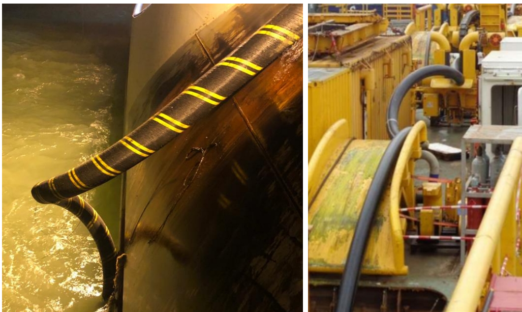
Figure 57: Examples of helical buckling (left: courtesy of TenneT, right: anonymous source, by permission)
