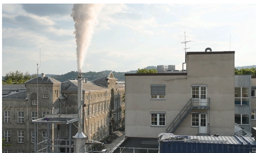
Fig. 5. CO 2 plume released during depressurization test 4.
