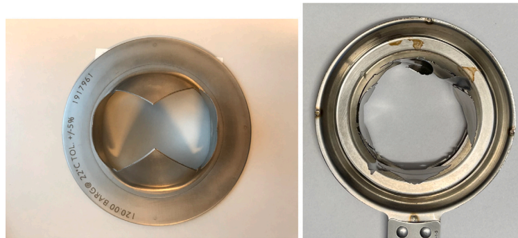
(a) X-scored rupture disk after test.
