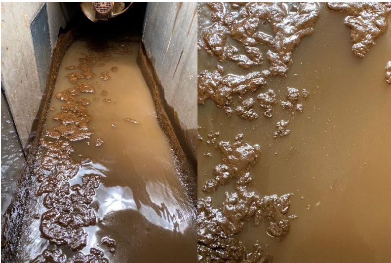
Figure 4-8: Emulsion 30 minutes after the second application of Dasic Slickgone NS.
