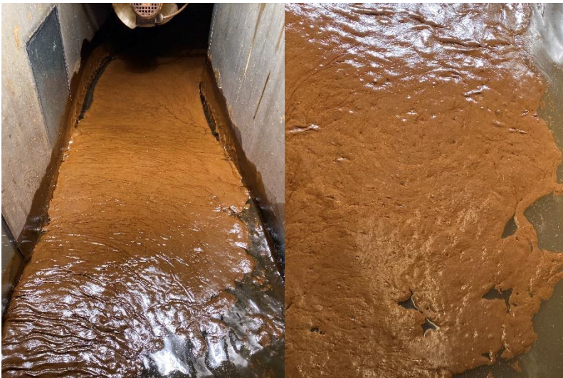
Figure 4-7: Emulsion 30 minutes after first application of Dasic Slickgone NS.
