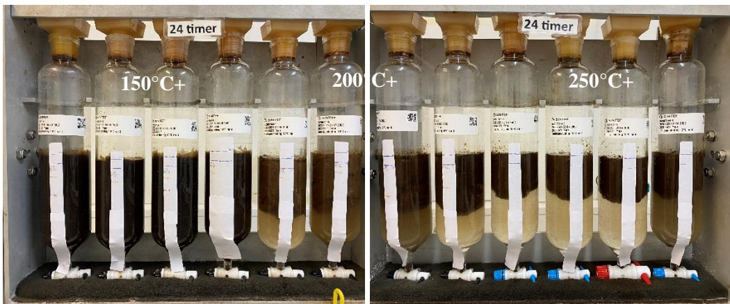
Figure 3-5: Rotating cylinders of water-in-oil (w/o) emulsions of Yme after 24 hours at 13 °C.
