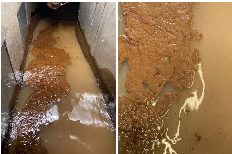
Figure 4-10: Emulsion 60 minutes after the third application of Dasic Slickgone NS.
