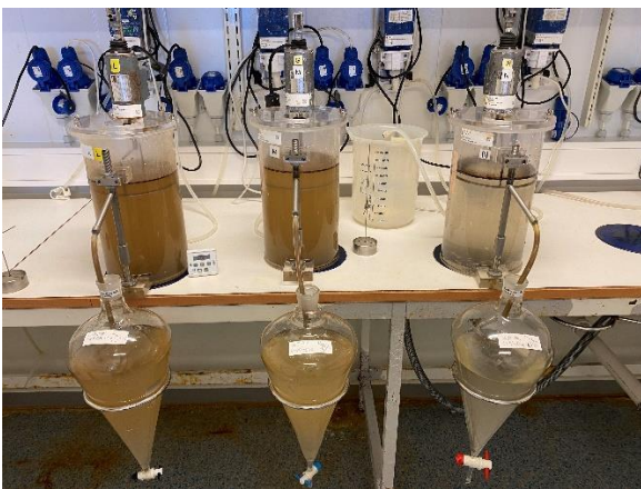
Figure 3-6: Example IFP-test on 200°C+ 50% emulsion, DOR/DER 1:25 of Yme. The two samples on the left are with Dasic Slickgone NS, and the one to the right is with Corexit 9500A.
