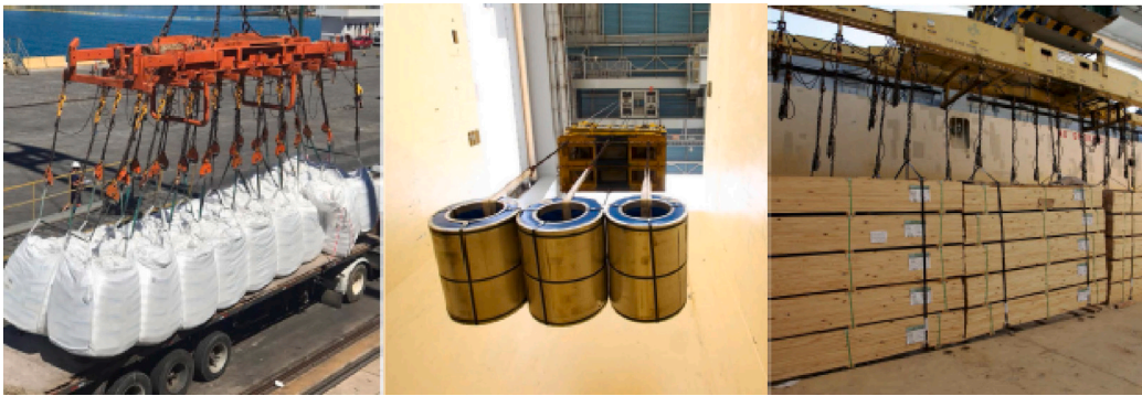
Fig. 4. Illustration of break-bulk cargoes and typical connection devices (left: Big bags, middle: steel coils, right: plywood). Source: Image credit: G2 Ocean.
