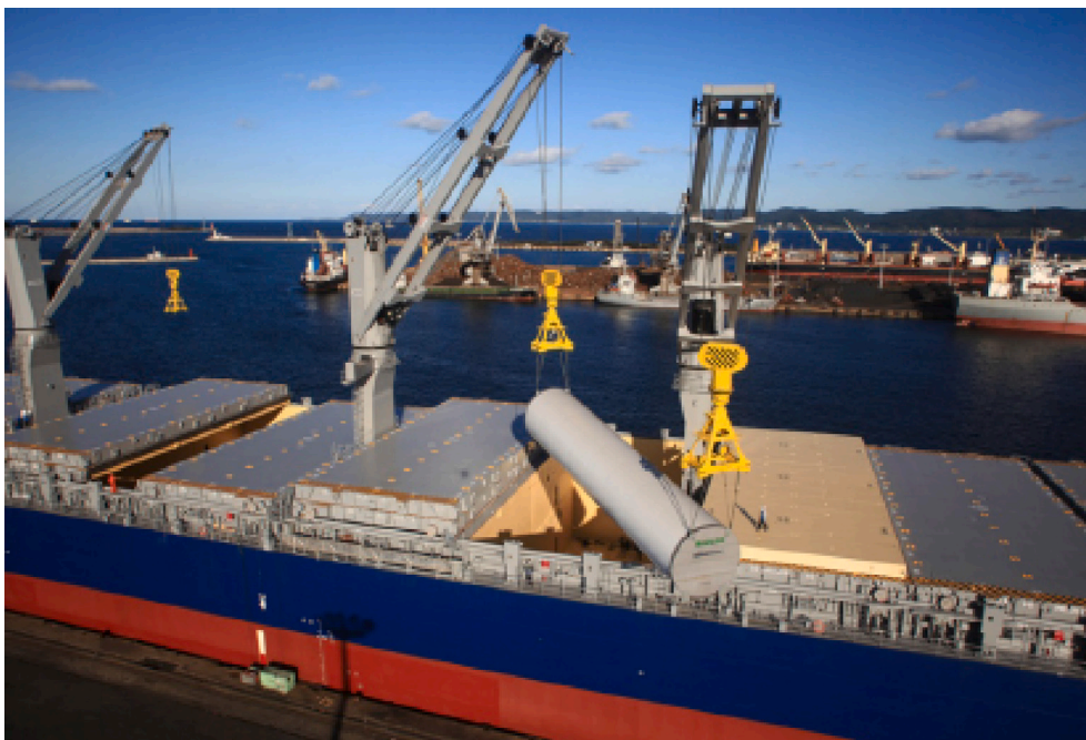
Fig. 1. Open hatch jib crane (wire-luffing crane) onboard a G2 Ocean ship. Source: Image credit: G2 Ocean.
