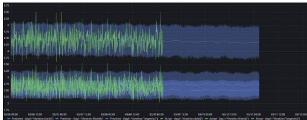
Figure 6. Actual and predicted values from Grafana ML for Vibration (Axial, Radial, Tangential) powered by PromQL.
