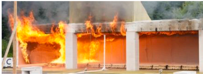
Fig. 18. During the first flashing wave, the heat exposure to the walls was sufficient to ignite the paper of the gypsum boards on the walls close by.
