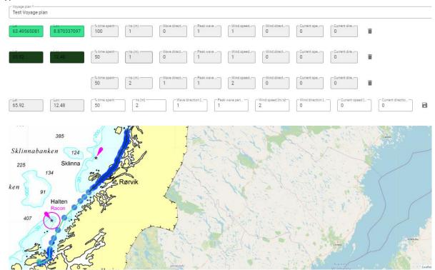
Figure 79: Route with weather configuration on two waypoints, one waypoint has two weather configurations
