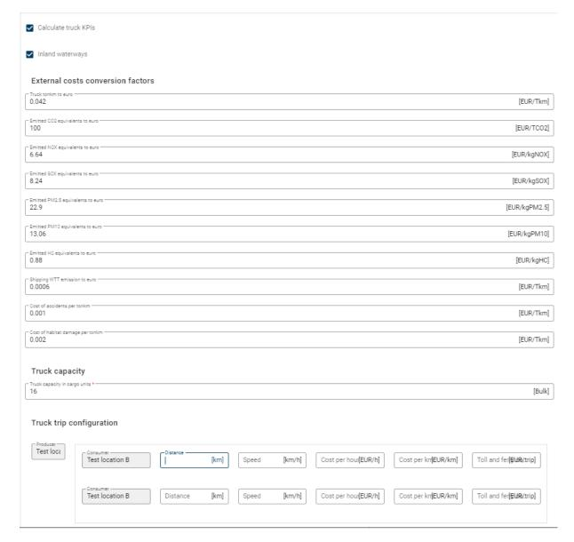
Figure 28: Truck comparison input parameter configuration
