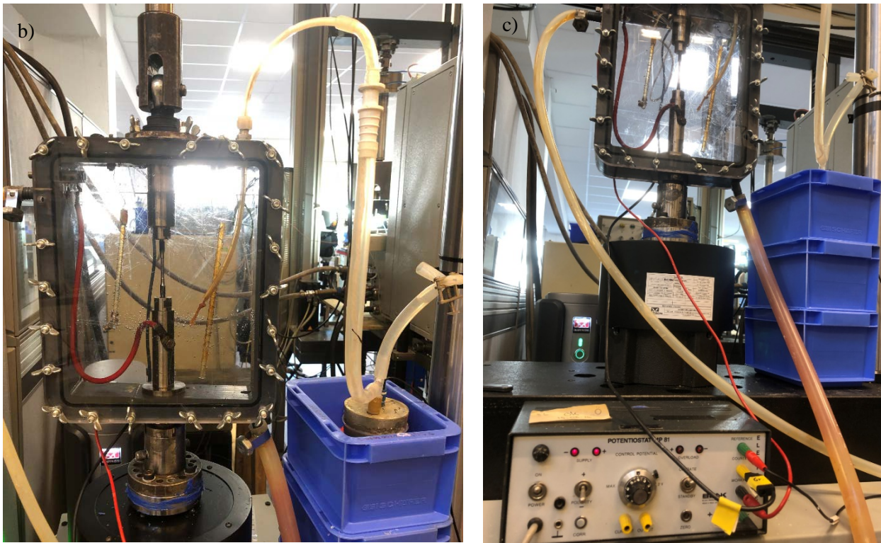
Fig. 23: a) Specimen geometry used for SSRT; b) Test set-up with mounted specimens and c) in-situ electrochemical hydrogen charging ongoing.
