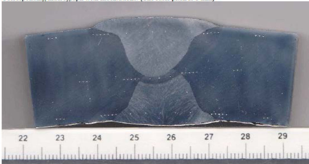
Corresponding macrograph with indentations. (The ruler pitch is 1 mm)
