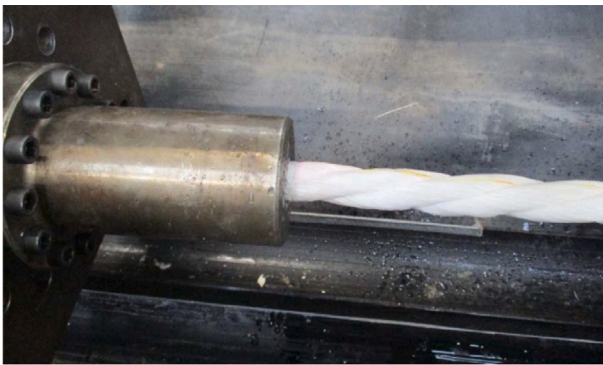
Fig. 4. Resin socket terminations were used to ensure the end termination did not reduce the break load or fatigue capacity. Photo provided by Tension Technology International.
