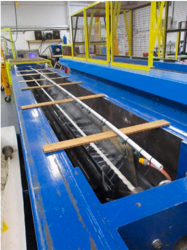
Fig. 3. Test bench for ropes. All ropes were soaked prior to testing, and water cooled throughout the test. Photo provided by Tension Technology International.
