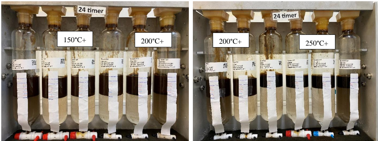
Figure 3-4 Rotating cylinders of water-in-oil (w/o) emulsions of Breidablikk after 24 hours at 5 °C.
