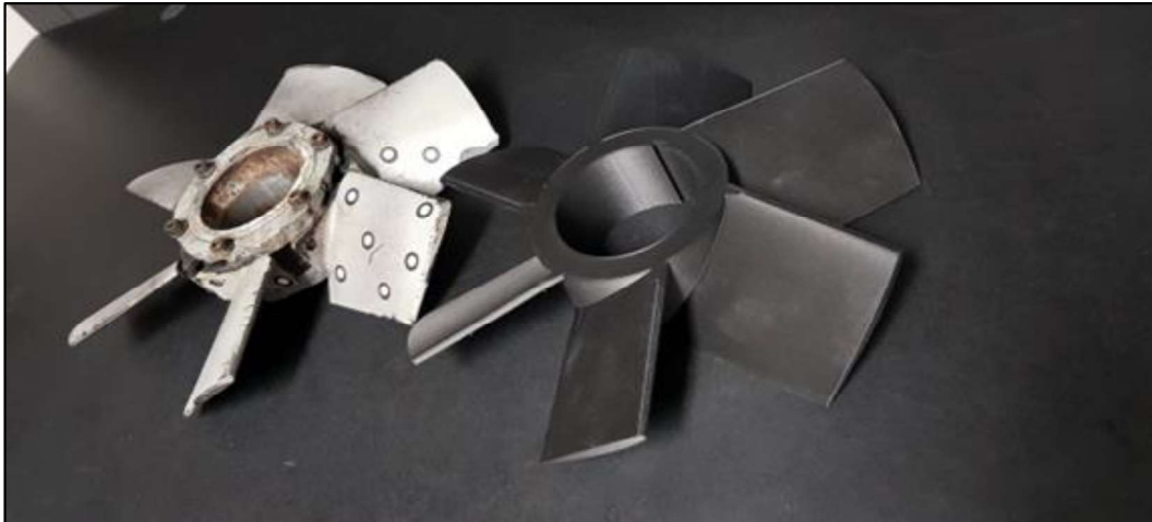
Figure 5: Fan for a motor and replacement part, made in the field by Fieldmade for Equinor during Trident Juncture 18. Since the original fan had gone out of production, reverse engineering and reproduction of this part was the only alternative to replacing the entire motor unit. Courtesy of Fieldmade and Equinor.
