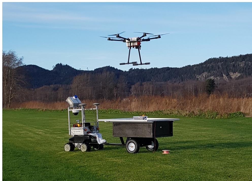
Figure 13. HEIFU UAS autolanding on an AGV-pulled charging station.
