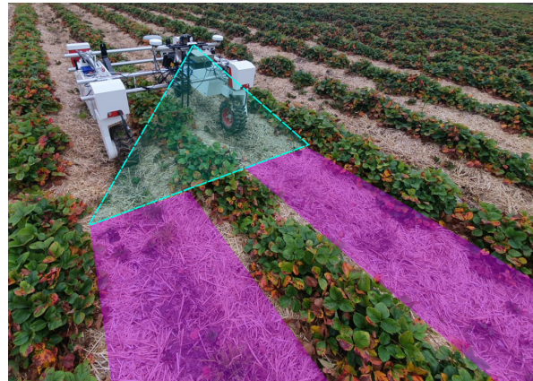
Fig. 1. The Thorvald II agri-robot platform operating in a strawberry field during data collection. We perform CNN-based segmentation to detect crop rows for visual guidance and propose an automatic labelling strategy for generating training data. During training, a mask representing crop locations is projected onto the camera image using the pose of the robot, measured with a dual-antenna RTK GNSS system. After training, CNN-based image segmentation can be used to guide the robot along the crop rows, without hand-drawn training labels.
