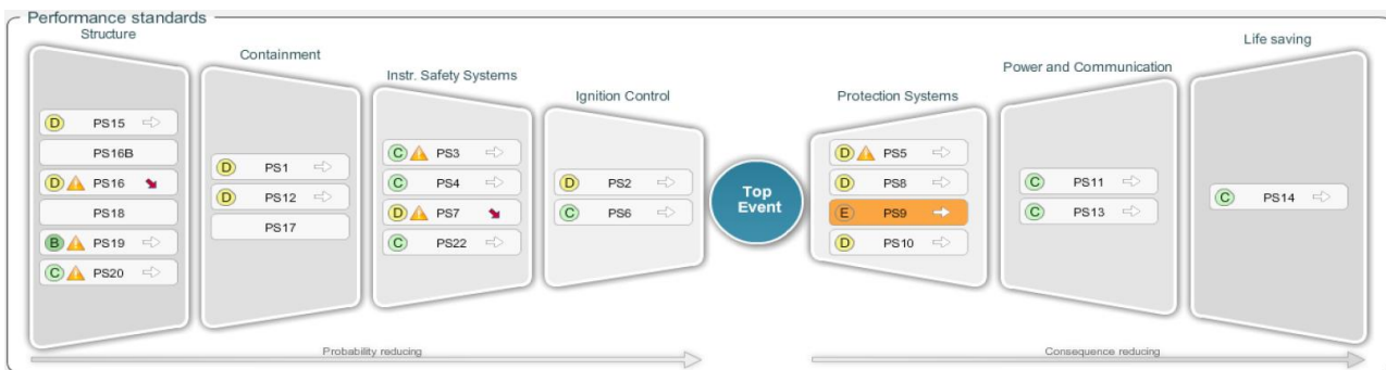
Figure 5.5 Statoil's TIMP visualization of technical barrier status (/9/)
