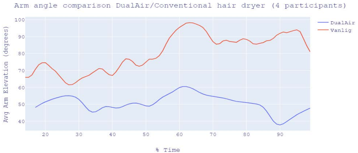
Figure 10 Shoulder angles for periods of use of Dual Air and a conventional hairdryer. Higher during use of conventional hairdryer during similar techniques. Data from 4 participants.
