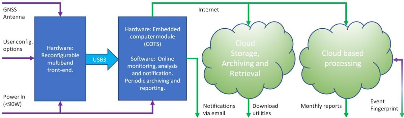
Fig. 2. ARFIDAAS high level functional diagram showing interfaces
