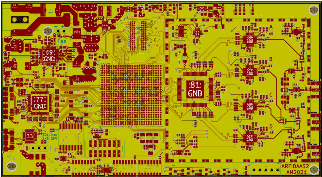
Fig. 1. ARFIDAAS second generation front-end printed circuit board (13.5 x 7.5 cm)
