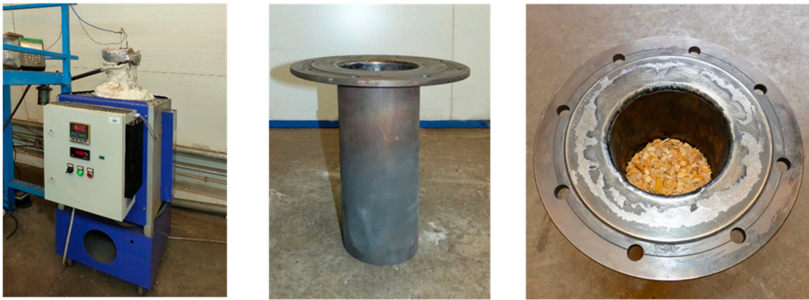
Figure 1. The electric resistance furnace and the steel retort loaded with biomass.
