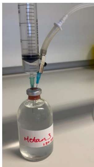
Figure 5: Sample removal and replacement with nitrogen.
