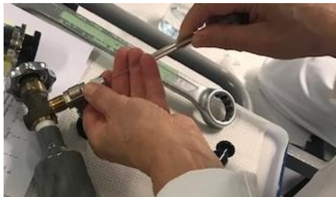
Figure 4: Transfer of ^{13}\text{CH}_4 from lecture flask to gas-tight syringe
