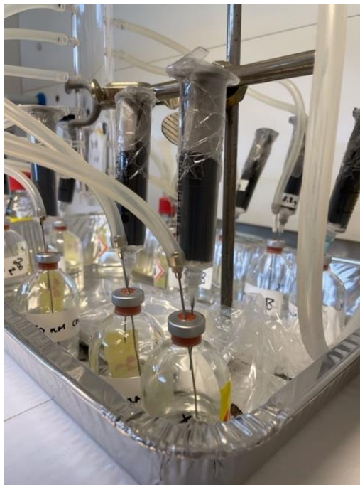
Figure 12: Sparging of samples and trapping of radioactive material in headspace in columns with activated carbon.
