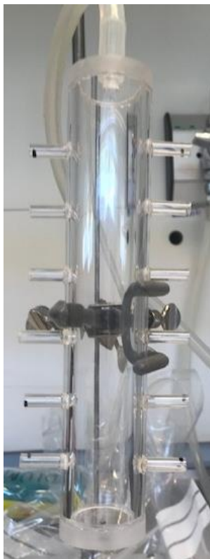
Figure 11: Unit for sparging of samples with N 2 gas before analyses
