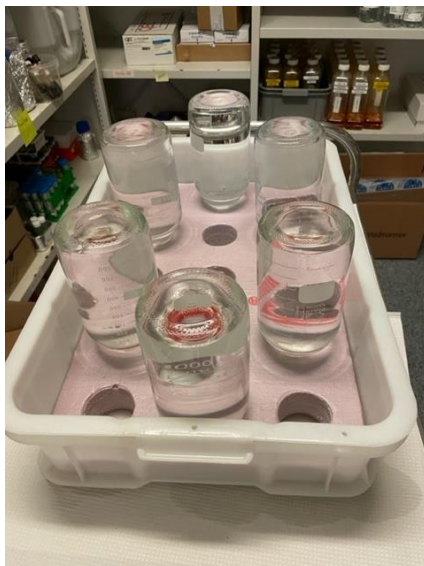
Figure A.3: Incubation of 1-L flasks upside down.
