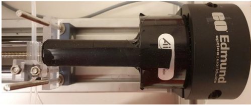
The LED array and tube directing light towards the imaging cuvette.
