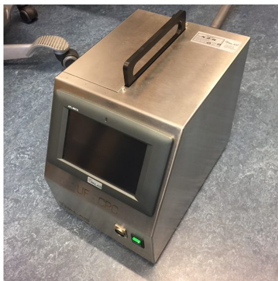
Figure 5.2 Palas UF-CPC 200 condensation particle counter applied during the Tiller pilot test campaign
