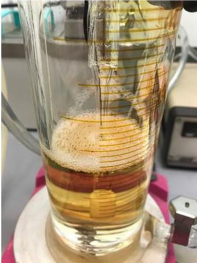
Lean 30% MEA foam did not collapse completely
