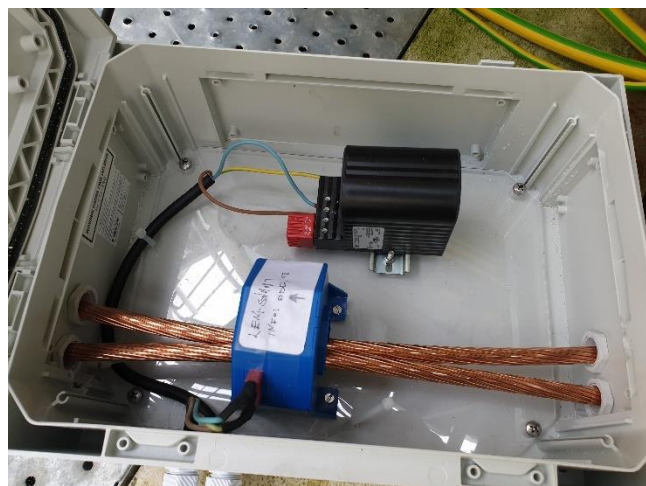
Figure 3-2: Neutral of transformer thread through a regular hall effect sensor (blue). Also a heater (black).
