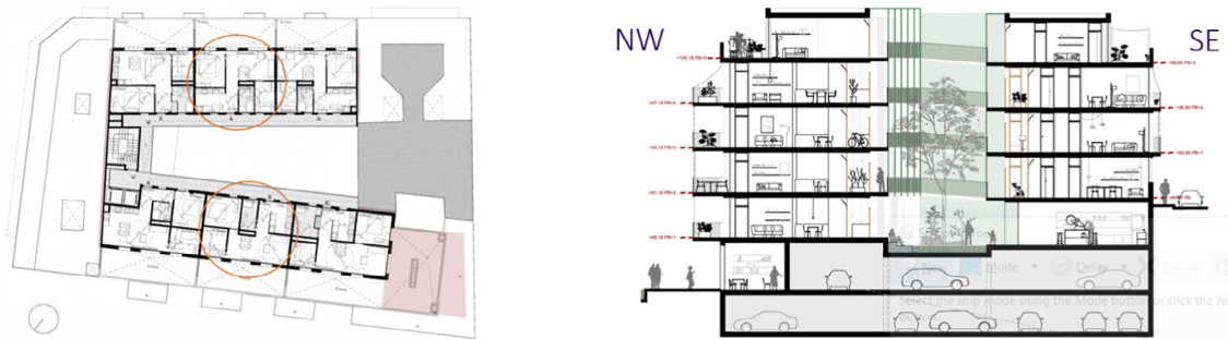
Fig. 4. Architectural drawings of the floor plan of the Barcelona demo site building's attic floor (left) and the elevation section (right). Apartments that were modelled in detail are circled with orange. (For interpretation of the references to colour in this figure legend, the reader is referred to the web version of this article.)
