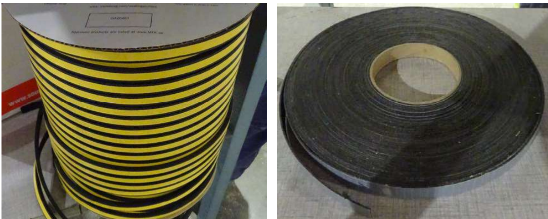
Figure 3-6 Glazing gasket (left) and intumescent strip (right)
