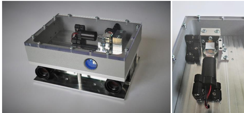
Fig. 10. (Left) Assembled 3D camera. The interferometric projector is mounted on top, while two cameras forming a stereo pair, as well as control electronics are mounted below. (Right) Close-up showing the interferometer. The laser is shown at the bottom, beam splitter in the center, movable mirror on top, reference mirror to the left and expansion lens to the right.
