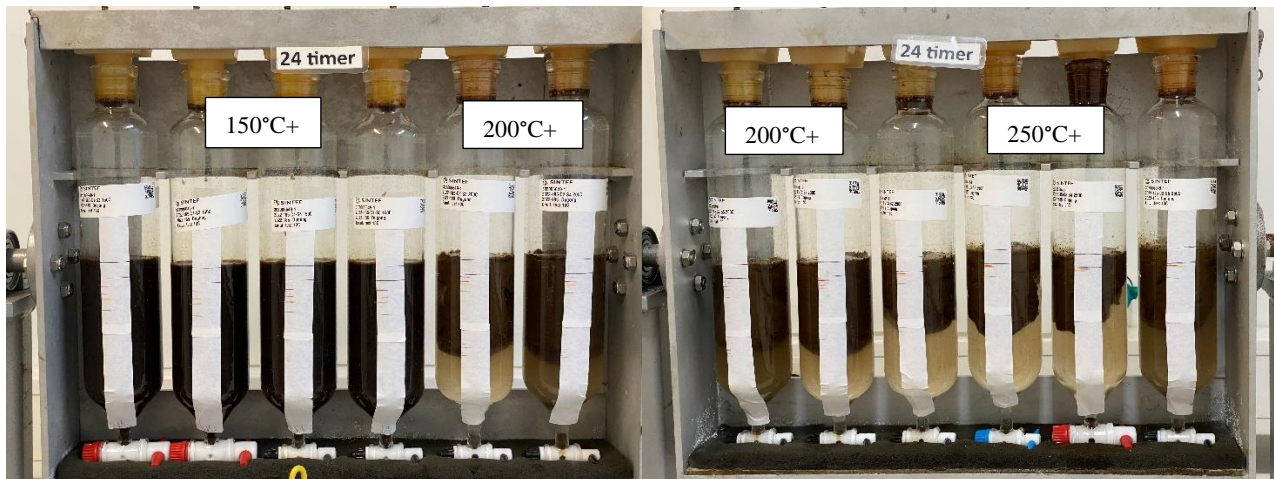
Figure 3-4 Rotating cylinders of water-in-oil (w/o) emulsions of Dugong after 24 hours at 13 °C.
