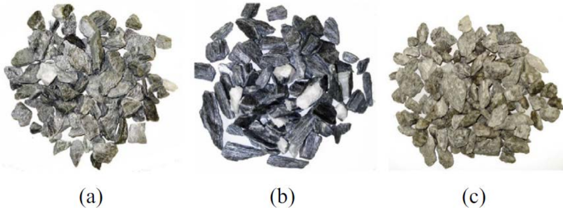
Figure 10: Aggregates used in concrete mixes by Voit and Zimmermann [47]. (a) quartz phyllite, (b) schist, (c) central gneiss.
