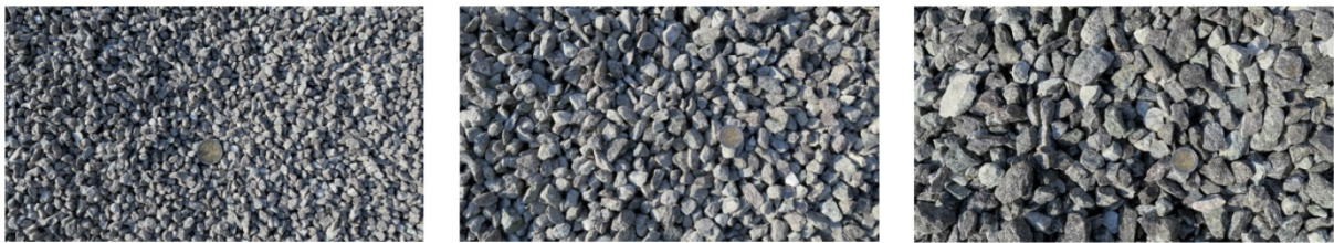
Figure 24: Fractions 3/8 mm, 8/16 mm and 16/32 mm [46].
