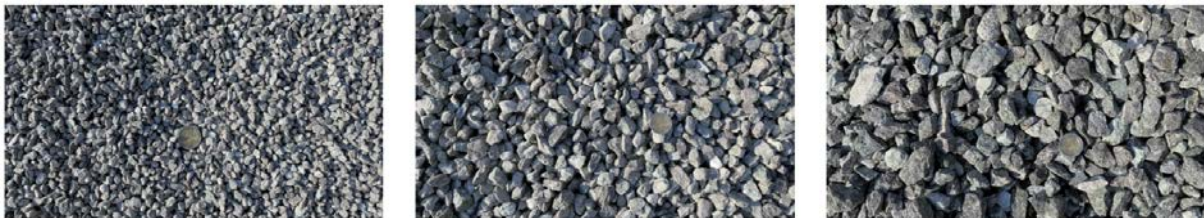
Figure 8: Fractions 3/8 mm, 8/16 mm and 16/32 mm [46].
