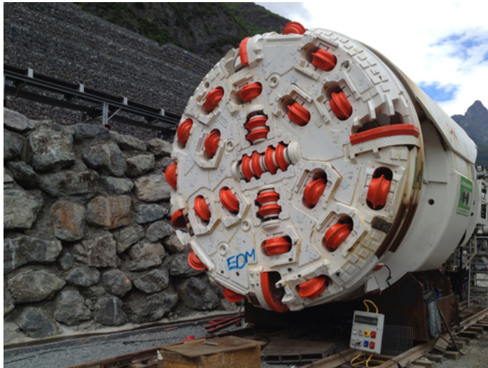
Figure 41: Tunnel Boring Machine [90].
