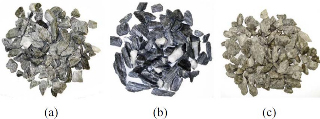
Figure 25: Aggregates used in concrete mixes by Voit and Zimmermann [47]. (a) quartz phyllite, (b) schist, (c) central gneiss.
