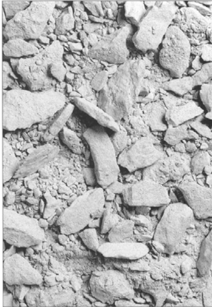
Figure 6: TBM material from Polmengo tunnel [40].
