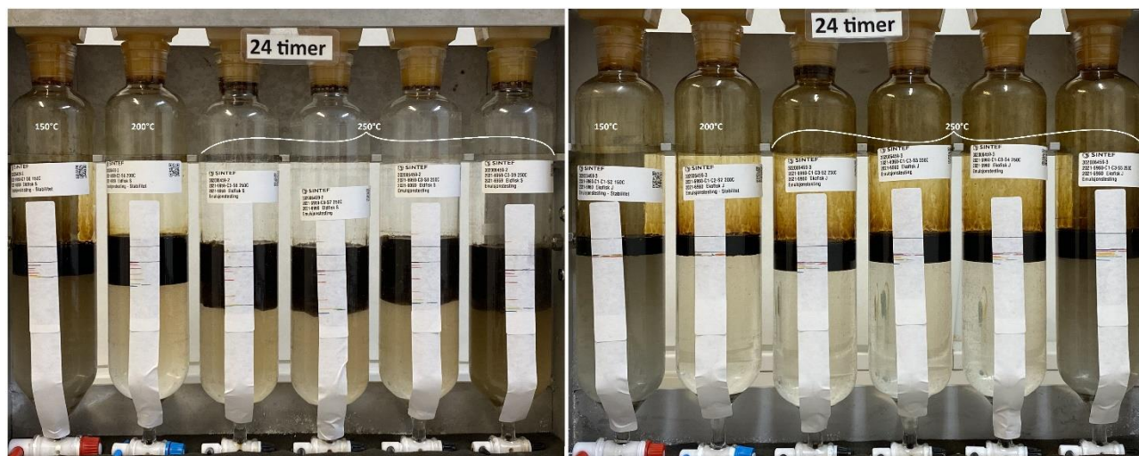
Figure 7-2 Rotating cylinders containing Eldfisk S (left) and Ekofisk J (right) after 24 hours of rotation at 13 °C. The Ekofisk J 2021 contains production chemicals and show lower degree of emulsification than expected for similar oil without prod. chemicals.
