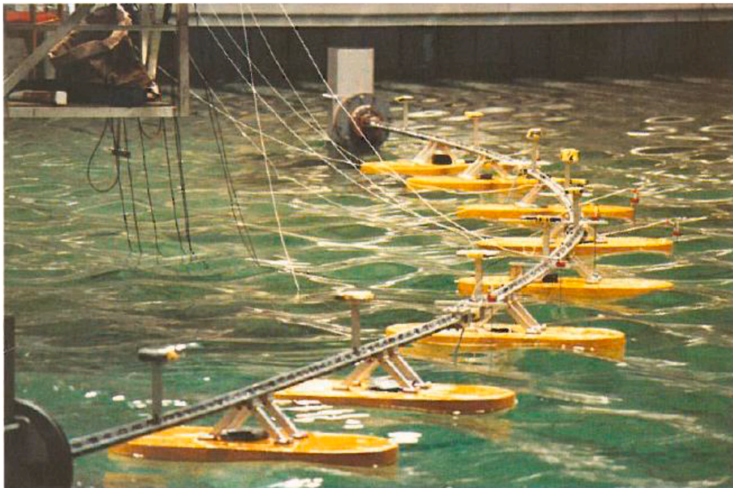
Fig. 1. Hydroelastic bridge model at MARINTEK [Xiang and Løken, 2019].
