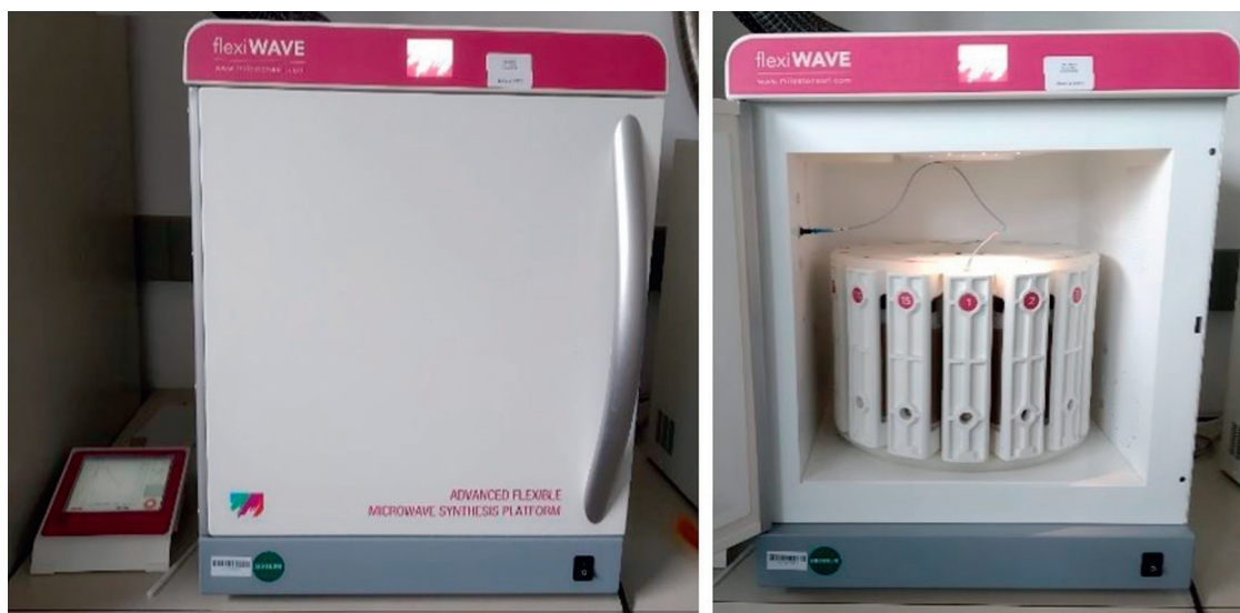
Fig. 13. MW system at the VITO laboratory used for leaching process
