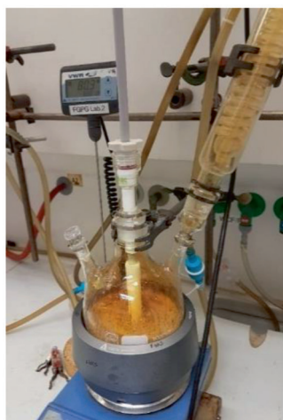
Fig. 3. Up-scale of VUT's leaching process (100 g catalyst)
