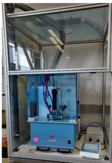
Fig. 17. VITO's litre-scale pressure-sealed MW leaching system with anticorrosion hybrid configuration (synthWAVE/ultraWAVE, Milestone Srl, Italy) in nitrogen-flushed confinement
