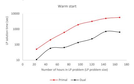
Figure 6: The LP solution time with warm start for varying LP-problem size. The black curve shows the results from the Dual Simplex method and the red curve shows the results from the Primal Simplex method. The vertical axis has a logarithmic scale.
