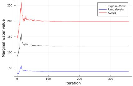
Figure 21: The evolution of the marginal water values per iteration for three selected reservoirs in week 1.
