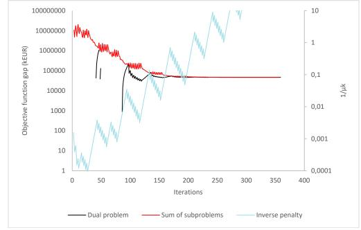
Figure 36: The evolution of the convergence gap and the inverse penalty of the LR solution process for parameter values from configuration 1.
