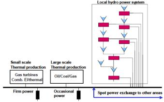
Figure 2: Model setup of a hydrothermal power system in a price area.
