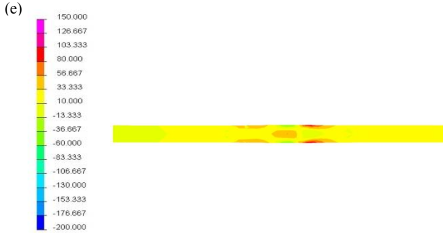
Fig. 10 Transverse residual stress distribution for welding (a) without and (b) and (c) with a Cu interlayer. Overall cross-section distribution of transverse residual stress for welding (d) without and (e) with a Cu interlayer.
