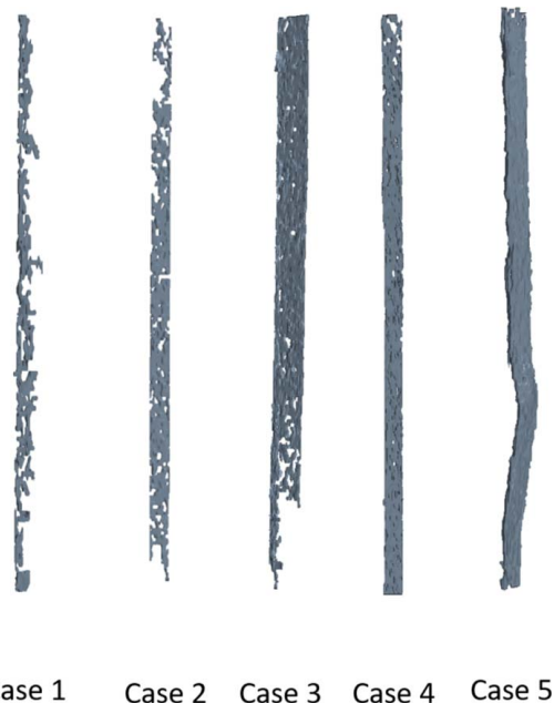
Fig. 2 Experimentally created geometries of radial cracks in cement sheath used in this study
