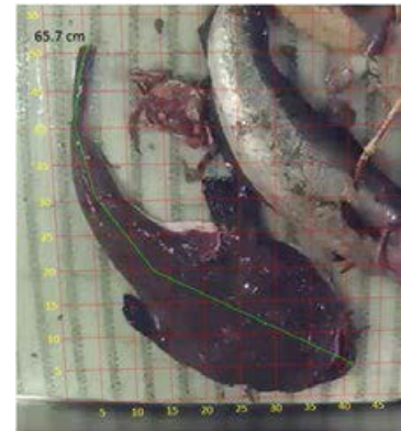
Figure 3: Example of image for video audit with grid overlay and measuring line integrated in the Black Box Analyzer set at measuring a monkfish ( Lophius piscatorius ) of 65.7 cm.
