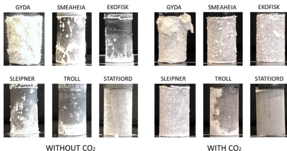
Figure 4. Images of graphite cathodes after polarization at 5 V, for 30 min in different reservoir waters with (right) and without (left) additional CO 2 .
