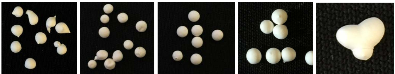
Figure 5: Different shapes of beads obtained for different concentration of calcium cations in the gelation bath: DWL-9-Ca0.2% (left), DWL-9-Ca0.5% (second) and DWL-9-Ca2.0% (middle). Tear-shaped beads and "triple-bead" of DWL-9-Ca10.0% (right).
