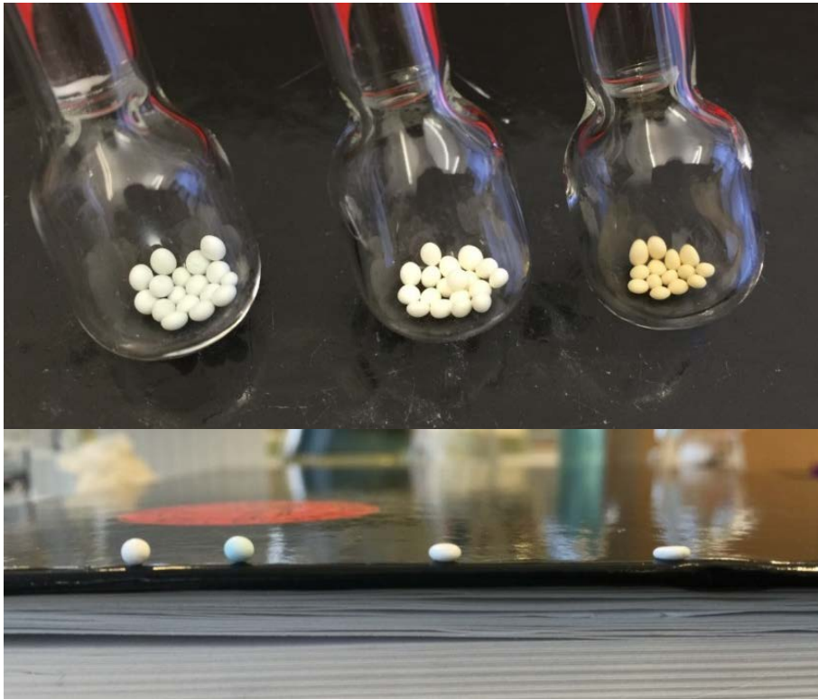
Figure 9: Top, from left to right: Cu-beads, Al-beads and Zr-beads. After activation at 120 °C for 2 hours under vacuum. Bottom, from left to right: Ca-bead, Cu-bead, Al-bead and Zr-bead.
