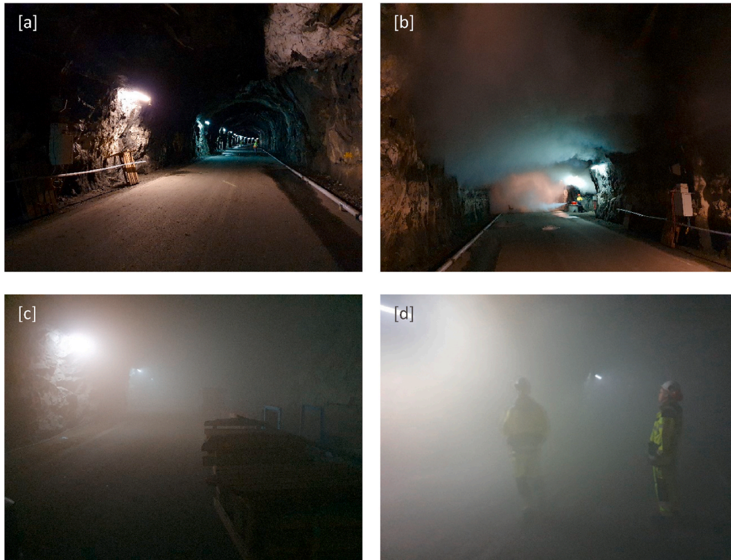
Fig. 5. Experimental setting depicting the Runehamar test tunnel used for Experiment 2 [a]; smoke machines filling up the tunnel [b]; gradual loss of vision product of the smoke [c]; and the perceptually limited vision in the tunnel to simulate evacuation conditions in a smoke-filled tunnel due to a fire [d]. Photos: Carl Södersten, SINTEF.
