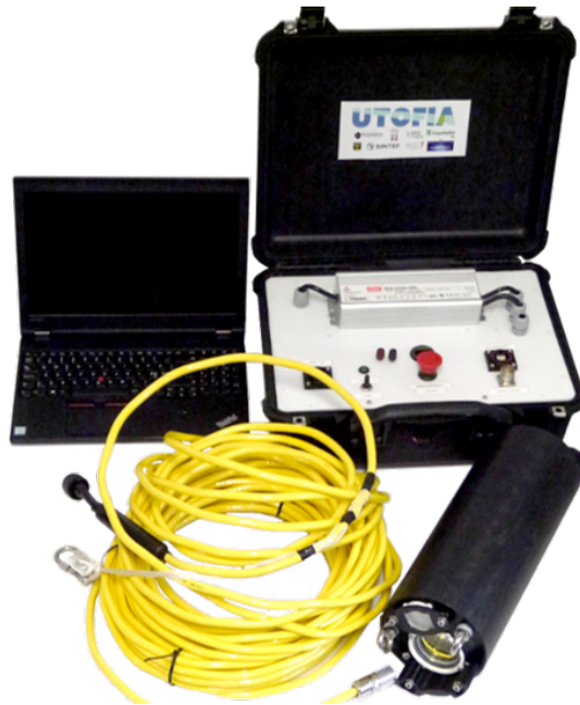
Figure 3. Range-gated 3D camera system. The full system includes a top-side box, Gigabit Ethernet cable, PC, and a cylindrical underwater housing.
