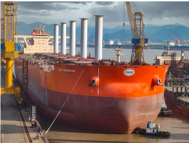
Fig. 1. Very large ore carrier (VLOC) M/V Sea Zhoushan of the Brazilian mining company Vale, equipped with five rotor sails.
