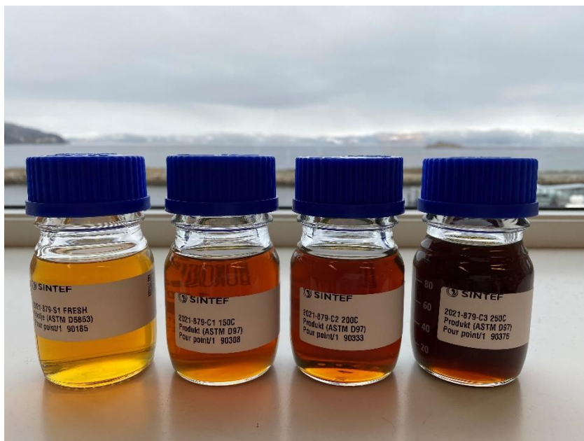
Figure 3-3 Utgard from left to right: Fresh oil, 150°C+, 200°C+ and 250°C+ residue.
