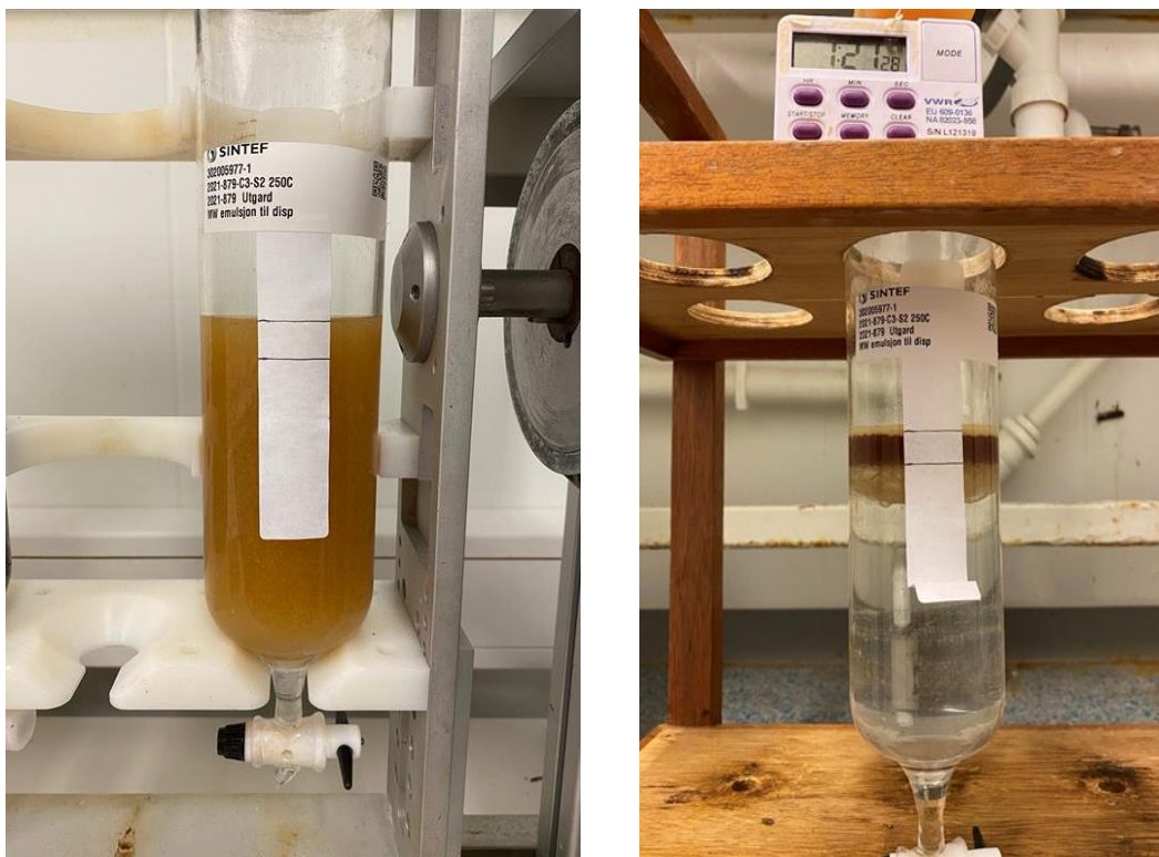
Figure 3-5 Left: Loose emulsion formation for 250°C+ residue of Utgard after 24 hours rotation time. Right: Released water from the 250°C+residue of Utgard within 1-hours stand still.
