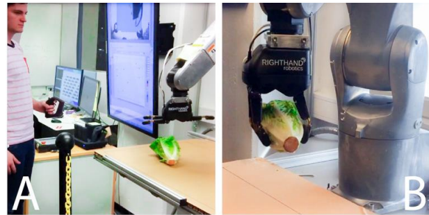
Figure 1. a) Learning from Demonstration : Teacher demonstrating grasps of compliant objects by remote control of the 6-DOF robot arm and gripper; b) Autonomous grasping : after learning the grasping skills from the teacher, the robot autonomously grasps compliant objects.
