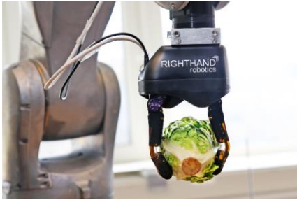
Figure 8. A snapshot of a close-up image of an autonomous robotic grasping of lettuce based on LfD learning policy.
