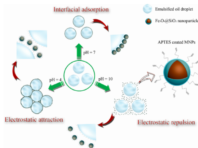
Figure 10. Schematic illustration of the interaction mechanism between APTES-coated MNPs and emulsified oil droplets. 139 Reproduced with permission from ref 139.
