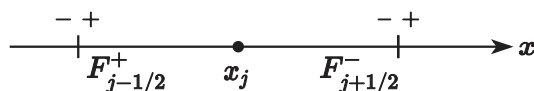
Fig. 3. The flux function \mathcal{F}_{j-1/2}^+ approximates the flux F_{j-1/2}^+ just to the right of the interface at x_{j-1/2} . The flux function \mathcal{F}_{j+1/2}^- approximates the flux F_{j+1/2}^- just to the left of the interface at x_{j+1/2} .
